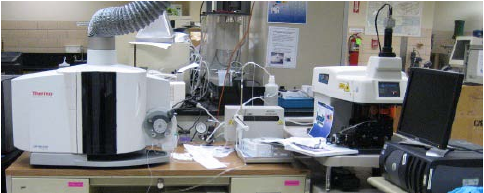
Thermo iCAP ICP-OES at the Library of Congress (Inductively Coupled Plasma – Optical Emissions Spectrometer)
